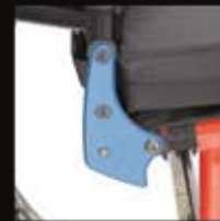
5 The back angle is adjusted simply by loosening a button-head screw and rotating an adjustment square located on the inside of this back bracket.
